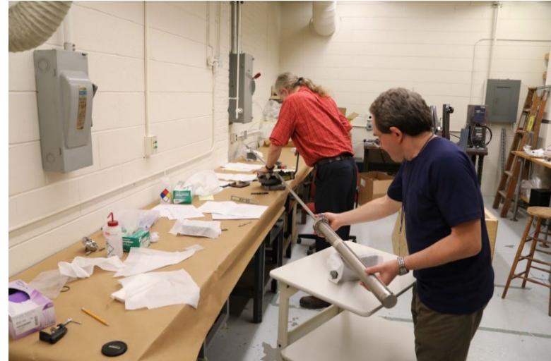
Tube bending and wiring
